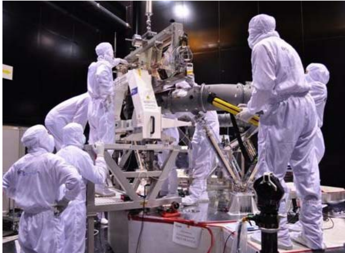
Alignment of the two telescopes in progress, tolerance 3 mm
